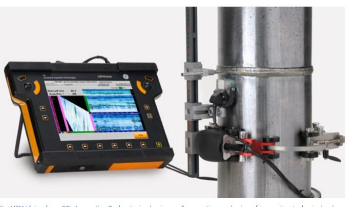
The USM Vision from GE's Inspection Technologies business allows optimum sharing of inspection tasks, is simple to operate and can remove the constraints associated with radiography.
